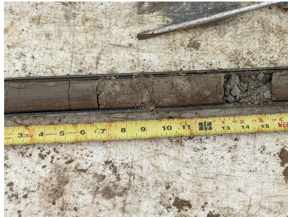
Figure 2- Transition from brown silt and sand to heavily compacted Gray sand found in the bottom 5 ft of boring B-1.
